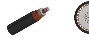
PVC/LSOH outer sheath Plain annealed copper metallic screen XLPE/EPR insulation Extruded semi-conducting insulation screen Extruded semi-conducting conductor screen Plain circular compacted aluminium conductor
